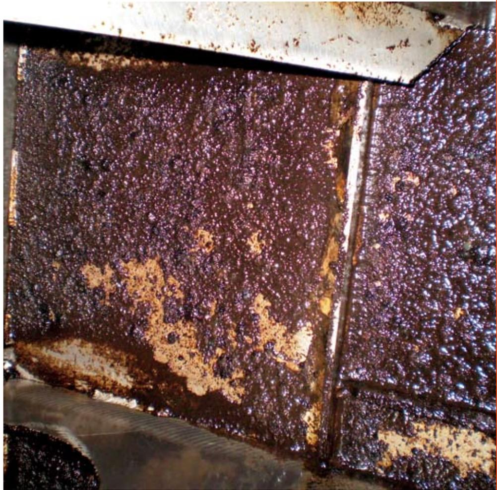
**M**ost boat owners are aware that the diesel bug micro-organism can grow inside the fuel tank, feeding on the diesel fuel itself, especially if the vessel isn't used much.
